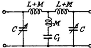
FIG. 4.8b.—Combined Mutual Inductance and Shunt Capacitance Coupling.
