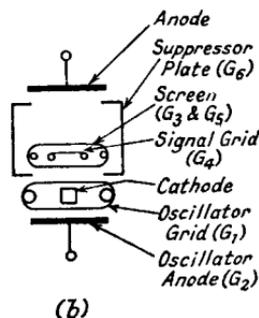
FIG. 5.8b.—An Improved Pentagrid Type of Frequency Changer.
