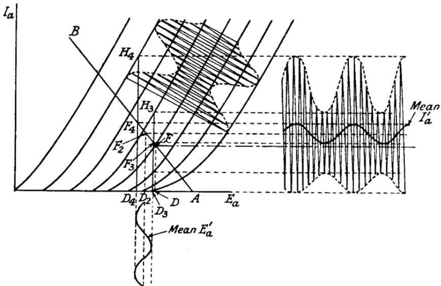
FIG. 8.18c.—Anode Bend Detection, with Anode Bypass Capacitance, referred to the  $I_a E_a$  Characteristic.
