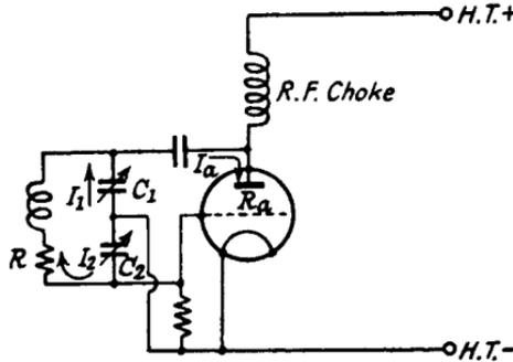
FIG. 6.5.—The Colpitts Oscillator.
