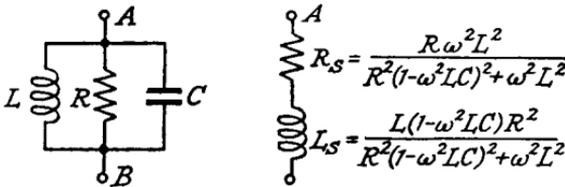
FIG. 1A.3.—A Parallel Circuit and its Series Equivalent.
