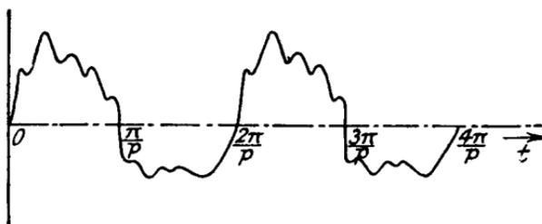
FIG. 2A.1.—An Example of a Periodic Wave which can be resolved into its Components by Fourier Analysis.
