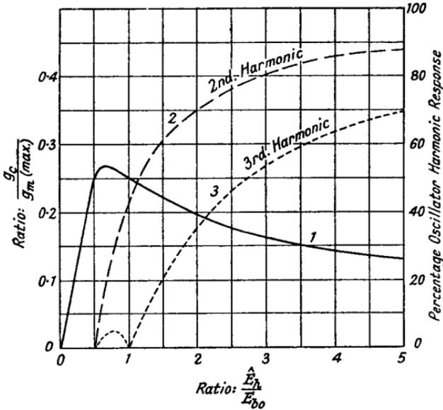
FIG. 5.11a.—Conversion Conductance and Oscillator Harmonic Response Curves for the Normal Type of Frequency Changer with Linear Mutual Conductance Characteristic.
