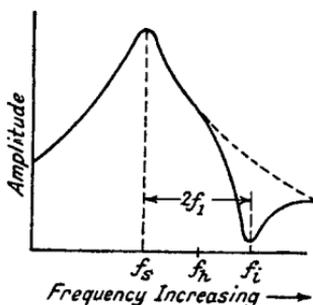
FIG. 5.20.—The Required Selectivity Curve for the R.F. Circuits preceding the Frequency Changer.
