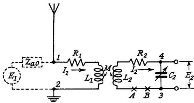
FIG. 3.8a.—An Aerial Circuit with Mutual Inductance Coupling.
