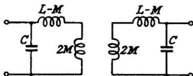
FIG. 7.4a.—Mutual Inductance Coupling with the Circuits Separated.
