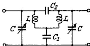
FIG. 4.8a.—Combined Series and Shunt Capacitance Coupling.
