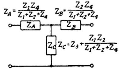
FIG. 3.16c.—The T Network Equivalent of Fig. 3.16b.
