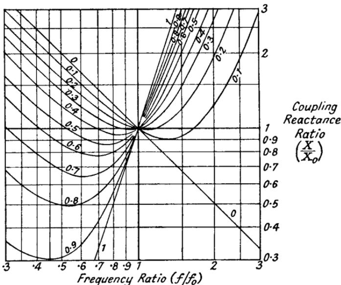
FIG. 4.13.—The Variation of Reactance Ratio Against Tuning Frequency Ratio for Combined Shunt and Series Capacitance Coupling.
