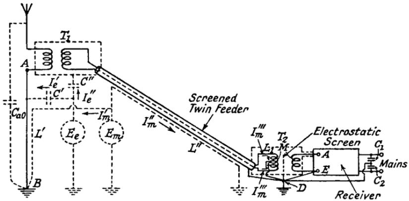
FIG. 3.20.—A Local-Interference Reducing Aerial System.
