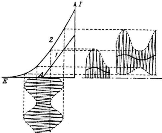
FIG. 8.1.—Detection with Linear (1) and Parabolic (2) Characteristics.
