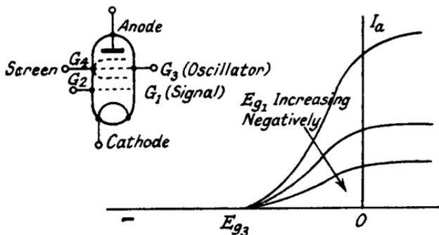
FIG. 2.10.— $I_a E_{g_3}$  Curves for a Hexode Valve with Different Signal Grid Bias Voltages.
