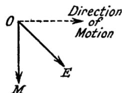
FIG. 3.2b.—A Horizontally Polarized Wave.
