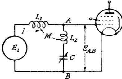
FIG. 5.21.—The Equivalent Circuit for the Tapped Coil Image Suppressor.
