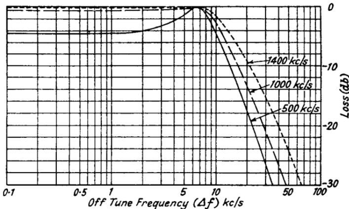
FIG. 4.10.—Selectivity Curves for a Tunable Band-Pass Filter.
