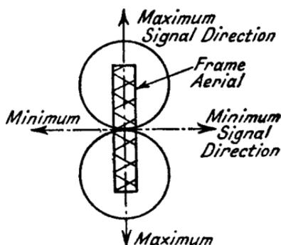
FIG. 3.7b.—The Directional Diagram of a Frame Aerial.
