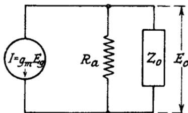
FIG. 2.12b.—The Valve as a Constant Current Generator.
