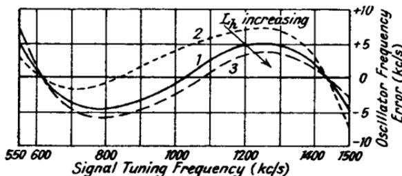
FIG. 6.19.—Calculated Error Curves for Three-point Ganging.
