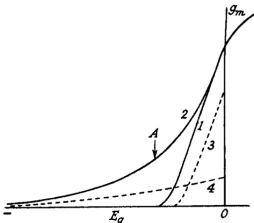
FIG. 2.8.— $g_m E_g$  Curves for a Tetrode or Pentode Valve.
