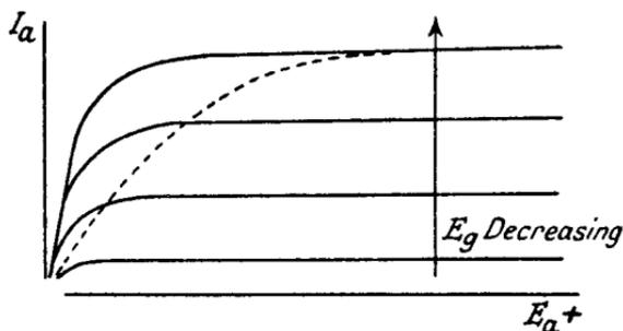
FIG. 2.7.— $I_a E_a$  Curves for a Pentode Valve.
