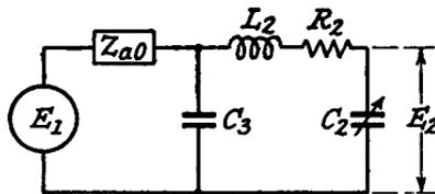
FIG. 3.12.—An Aerial Circuit with Shunt Capacitance Coupling.
