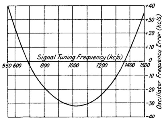
FIG. 6.17.—The Calculated Error Curve for Two-point Ganging.
