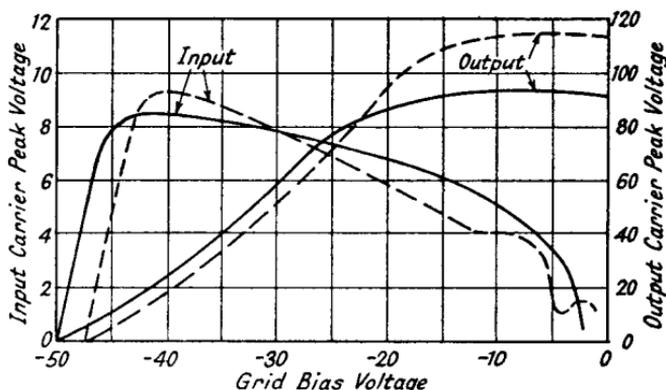
FIG. 5.16.—Typical Signal Handling Capacity Curves for Pentode and Hexode Frequency Changers.
