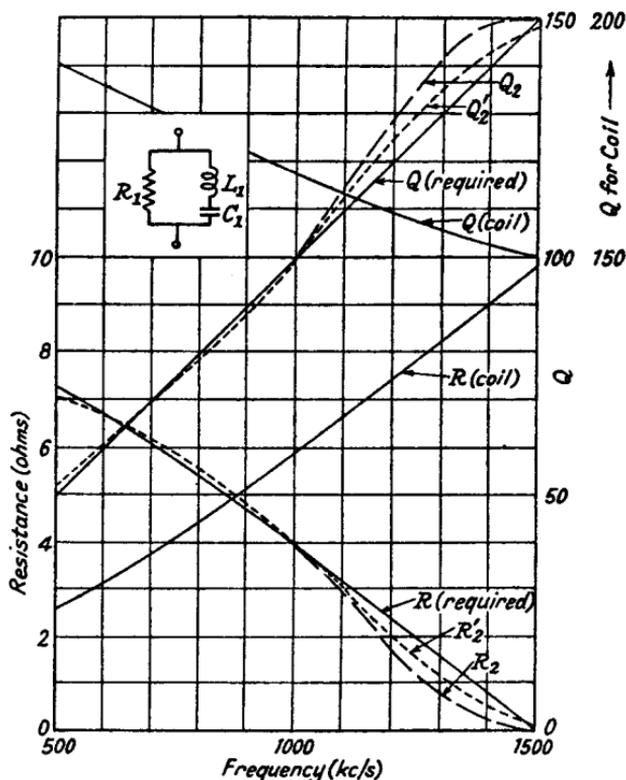
FIG. 4.4.—Correction Curves for a Tuned Circuit of Constant  $Q$  Value.
