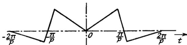
FIG. 2A.4.—A Wave Shape having Cosine Functions only.
