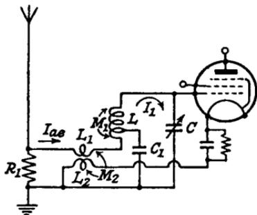
FIG. 5.23c.—Image Suppression by a Neutralizing Voltage Applied from the Aerial to the Cathode Circuit of the First R.F. Valve.
