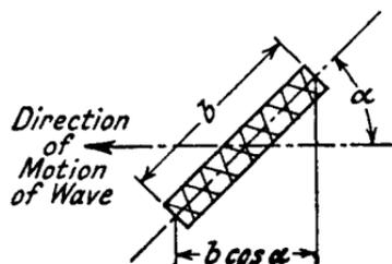
FIG. 3.7.a—Plan View of a Frame Aerial.
