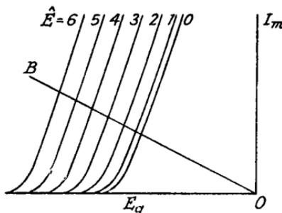
FIG. 8.23b.—Typical Curves for an Anode Bend Detector with Negative Feedback.
