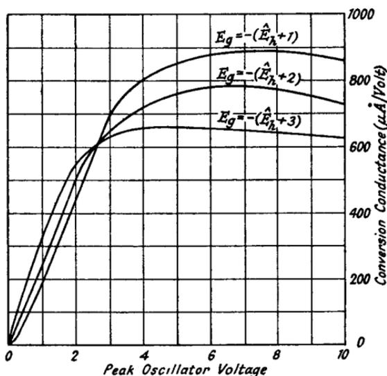
Fig. 5.1a.—Typical Conversion Conductance-Oscillator Voltage Curves for Signal and Oscillator Voltages in the Grid-Cathode Circuit.
