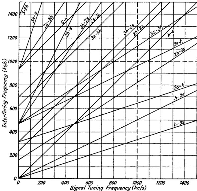
FIG. 5.9.—Interference Chart for an Intermediate Frequency of 465 kc/s.
