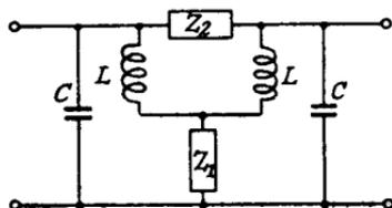
FIG. 7.1.—A Circuit with Combined Shunt and Series Coupling.
