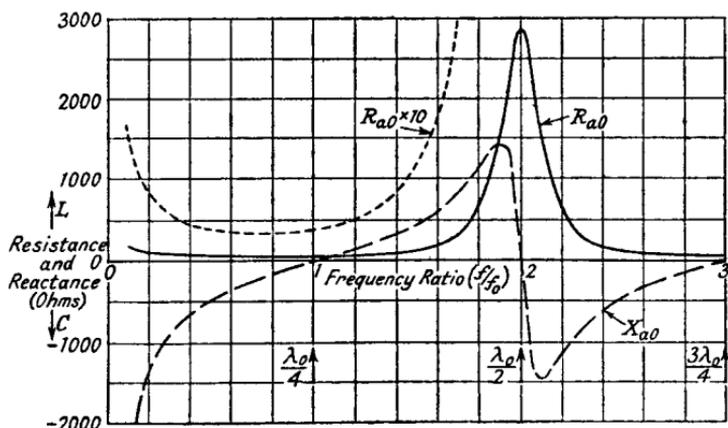
FIG. 3.4b.—The Resistance and Reactance Components of the Terminal Impedance of a Vertical Aerial having a Quarter Wavelength Radiation Resistance of 40 Ohms.
