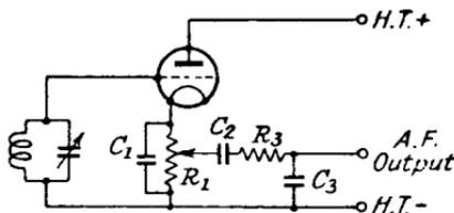
FIG. 8.23a.—The Anode Bend Detector with Negative Feedback.
