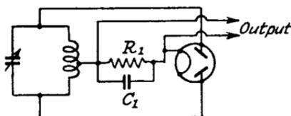
FIG. 8.22.—Double Wave Detection with a Diode.
