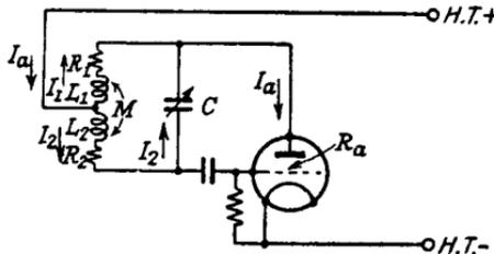
FIG. 6.4.—The Hartley Oscillator.
