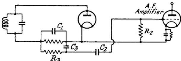
FIG. 8.5.—A Diagram of Connections for the Coupling from a Diode Detector to an A.F. Amplifier.
