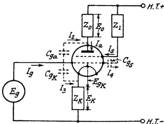
FIG. 2.13.—A Circuit showing Coupling to the Grid by Interelectrode Capacitance.
