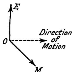
FIG. 3.2a.—The Representation of a Vertically Polarized Wave.
