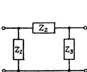
FIG. 3.15b.—An Unsymmetrical  $\pi$  Section.
