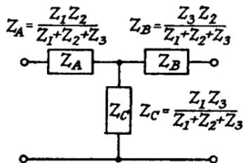
FIG. 3.15c.—The T Network Equivalent of Fig. 3.15b.
