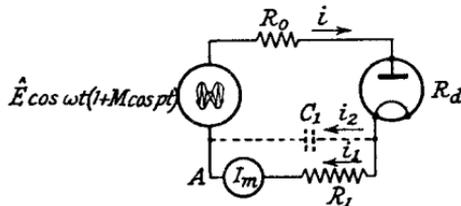
FIG. 8.2.—A Diode Detector.
