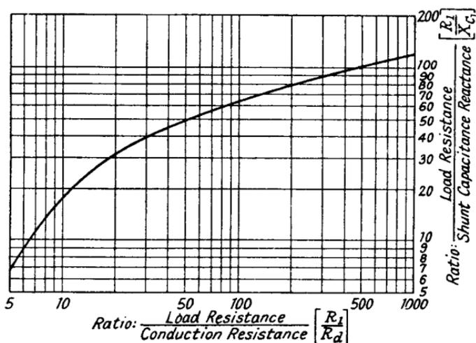
FIG. 8.13b.—A Curve of Load Resistance to Shunt Capacitance Reactance Ratio against Load Resistance to Conduction Resistance Ratio for Maximum Detection Efficiency.
