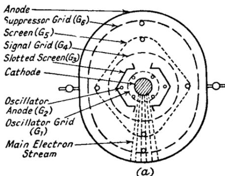
FIG. 5.8a.—The Electrode Structure of a Special Octode.
