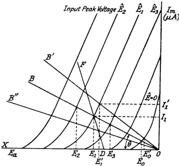
FIG. 8.4b.—Typical  $I_m E_a$  Curves for a Diode Detector.
