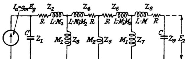
FIG. 7.11b.—The Equivalent Circuit for Two Loosely Coupled I.F. Transformers. [For  $Z_8$ , read  $L - M_1$  and  $R$ .]
