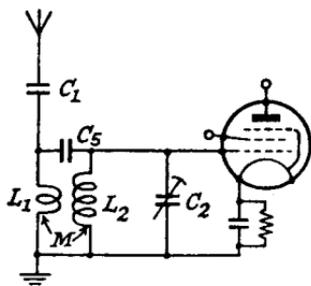
FIG. 5.24a.—Image Suppression on the Short Wave Band by Combined Mutual Inductance and Series Capacitance Coupling.
