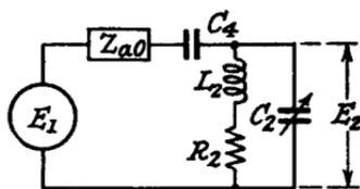
FIG. 3.14.—An Aerial Circuit with Series Capacitance Coupling.
