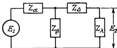
FIG. 3.10.—A Generalized T Network Coupling Circuit.
