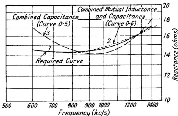
FIG. 4.12.—Required and Approximate Coupling Reactance-Frequency Curves.
