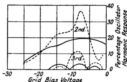
Fig. 5.15.—Typical Oscillator Harmonic Response Curves for a Pentode and Hexode Valve.
