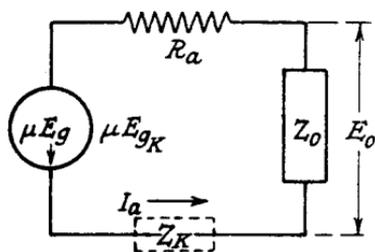
FIG. 2.12a.—The Valve as a Constant Voltage Generator.
