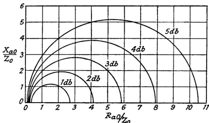
FIG. 3.22.—A Chart for Estimating Transition Loss due to Mismatching between an Aerial and Correctly Terminated Feeder.
