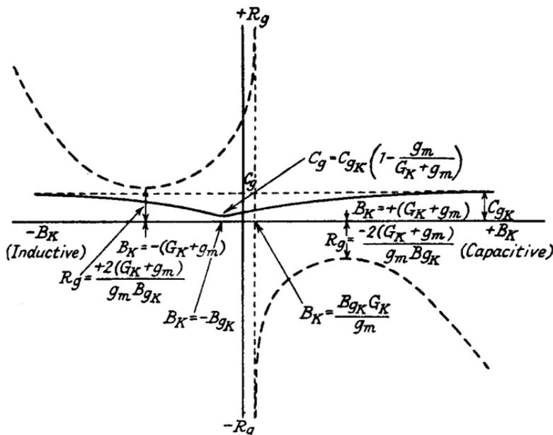
FIG. 2.16.—The Effect on Input Capacitance ( $C_g$ ) and Input Resistance ( $R_g$ ) of Varying Cathode Circuit Susceptance ( $B_k$ ).
