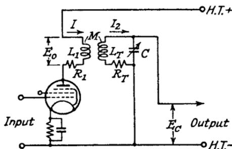
FIG. 4.7.—The Transformer Coupled Circuit.
