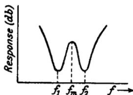
FIG. 7.13b.—The Frequency Response due to Cathode Feedback.
