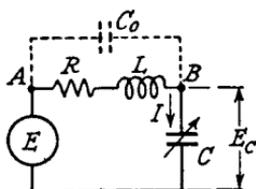
FIG. 4.1.—The Voltage Magnification of a Coil.
