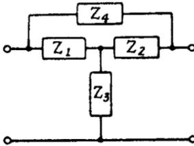
FIG. 3.16b.—An Unsymmetrical Bridged T Section.
