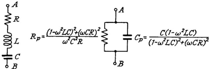
FIG. 1A.4.—A Series Circuit and its Parallel Equivalent.
