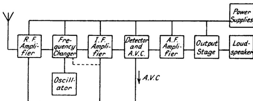
FIG. 1.8.—Schematic Diagram for a Typical Superheterodyne Receiver.
