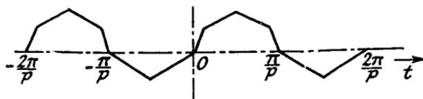
FIG. 2A.8.—A Wave Shape with Odd Sine and Even Cosine Functions.
