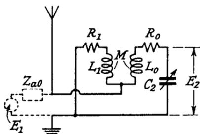
FIG. 3.13a.—Tapped Tuned Circuit Aerial Coupling.
