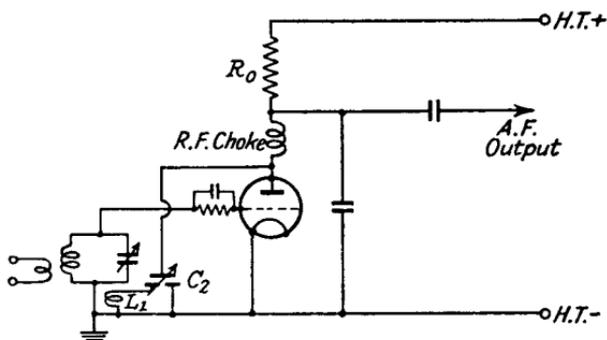
FIG. 8.20.—A Typical Circuit for a Regenerative Detector.
