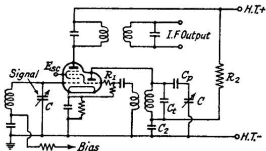
FIG. 5.6.—The Circuit for a Triode-Hexode Frequency Changer.
