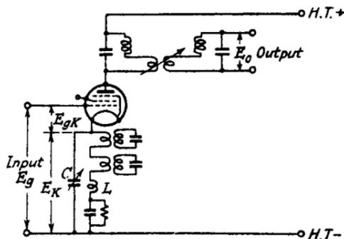
FIG. 7.13a.—An I.F. Amplifier with Cathode Feedback.
