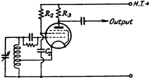
FIG. 6.11.—The Electron Coupled Oscillator.
