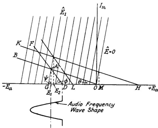
FIG. 8.6.—Ideal  $I_m E_a$  Curves for a Diode Detector showing the Effect of the Coupling Resistance  $R_3$  and Positive Bias.
