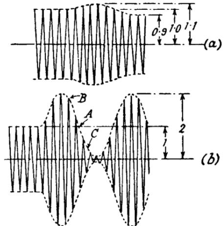
FIG. 1.1.—An Amplitude Modulated Wave.
