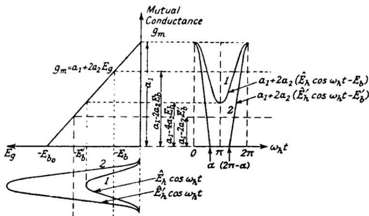
FIG. 5.10.—Linear Mutual Conductance Characteristic for the Normal Type of Frequency Changer.
