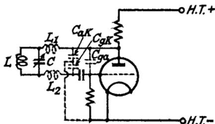
FIG. 6.14.—Parasitic Oscillation in the Modified Colpitts Oscillator.
