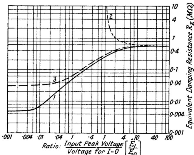
FIG. 8.11b.—Curves of Equivalent Damping Resistance against Voltage Ratio  $\frac{E_1}{E_0}$ .
