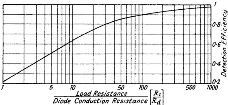
FIG. 8.8.—A Curve of Detection Efficiency against the Ratio of Load to Diode Conduction Resistance.
