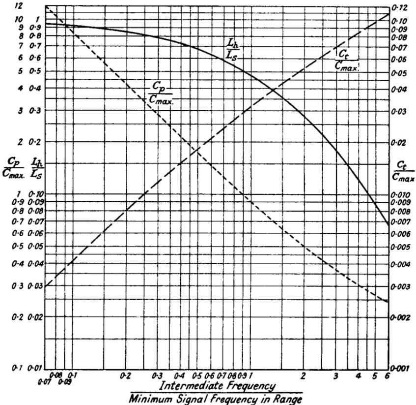
FIG. 6.21.—Curves for Ganging Component Ratios against Intermediate to Minimum Signal Frequency Ratios.
