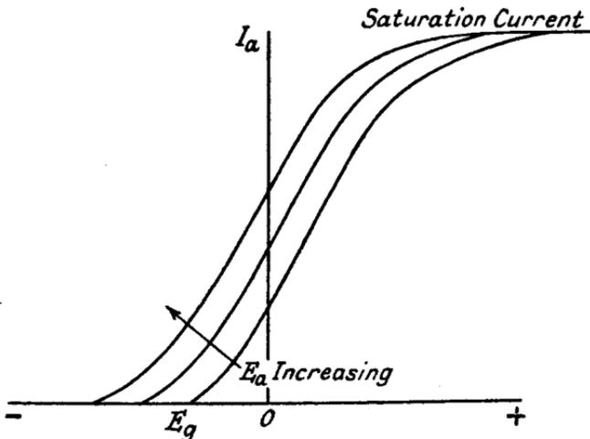
FIG. 2.4.— $I_a E_a$  Curves for a Triode Valve.
