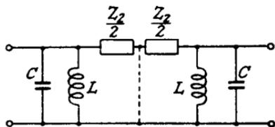
FIG. 7.3.—Separated Series Coupled Circuits.
